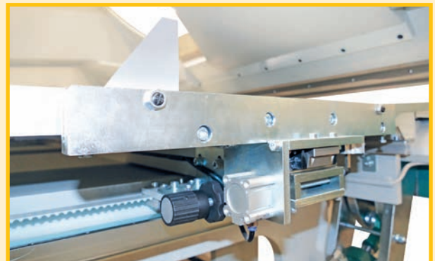
2 Pneumatic device for the back gauge's conicity
